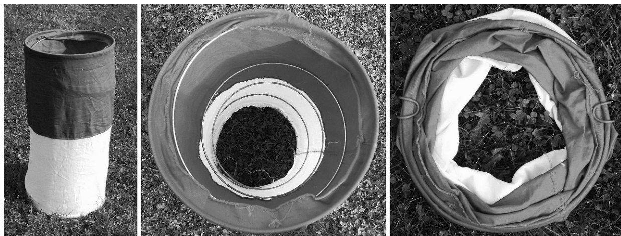
Fig. 1. The 700-g, collapsible cover cylinder developed to measure horizontal cover in the field measures 60 cm high x 30 cm diameter. The 30-cm upper section is red and the lower section is white (left photograph).
